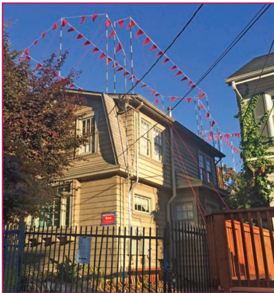
“Story poles” at 2718 Durant Avenue showing proposed height after remodeling. Anthony Bruce, July 2019.
